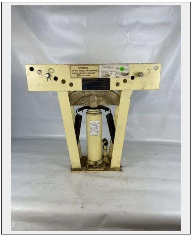
**Description**Hydraulic pipe bender with a 12-ton capacity.
