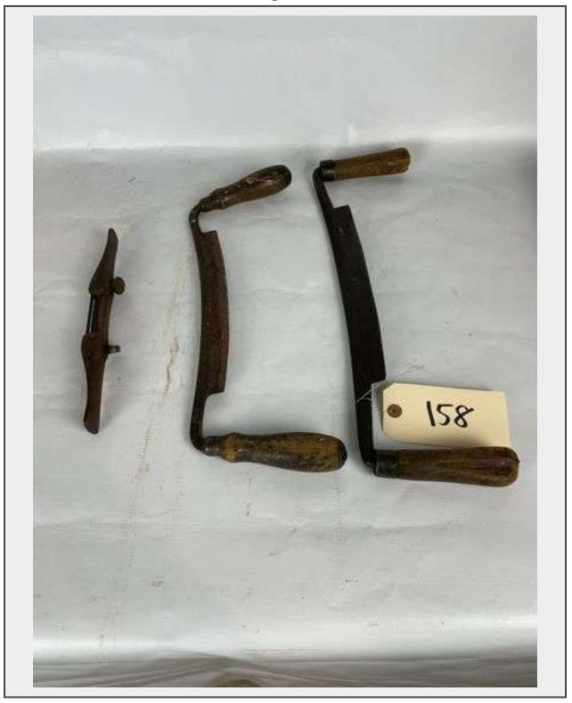
**Description**Includes two draw knives with wooden handles and an additional small woodworking tool.
